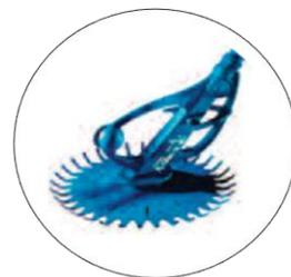
Suction cleaners are simple to install and are powered by the existing filter pump and plugged into the skimmer box. Acting rather like an underwater vacuum cleaner, the unit travels up the walls and across the floor. It travels in a random pattern, with the suction unit in contact with the surface of the pool lining. Dirt-laden water and debris is carried through a flexible hose into the pool filtration system.
